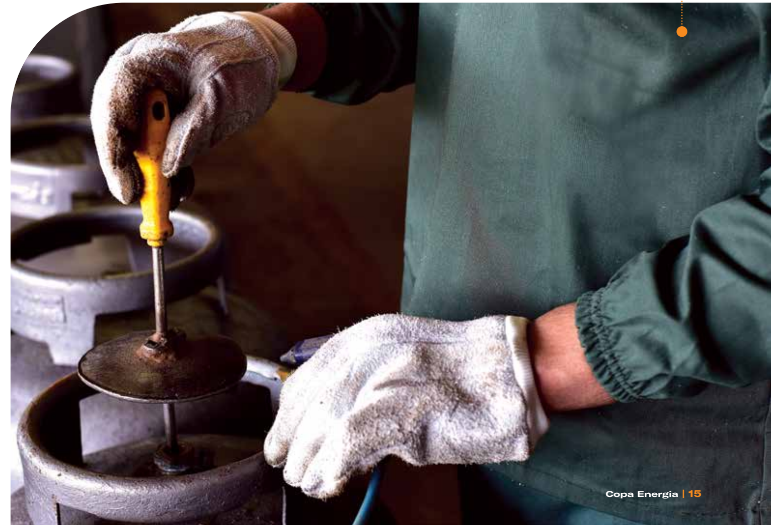
Operator adjusting leakage in the valve in the CO of Capuava.
